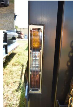
FLUSH MOUNTED LIGHTING
