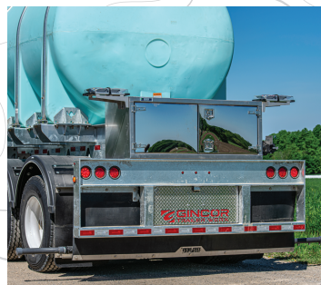
Cabinet Mounted Minibar lights, with 12' boom extension spray bar.
